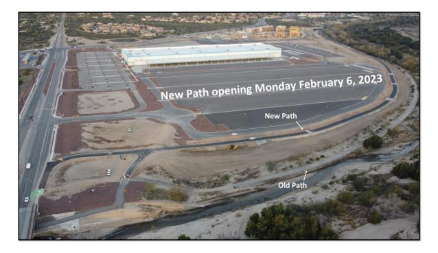
The contractor has finished installing new bank protection along with relocating a portion of the Loop pathway near the new Amazon facility north of Ina Road. The bank protection improvements provided the opportunity to raise a portion of the Loop pathway out of the Santa Cruz River flood zone, giving the public a safer more reliable walking and biking experience.
