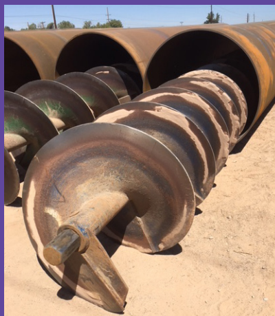
Below – Bore Pit and Tunnel for new piping; Right – Auger used during boring operations.
